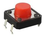
On/off electronic 12mm tactile switch that is only on when the button is pressed or if there is a definitive change in pressure. Used for circuit board, there are many different kinds of height for the switch knob, the standard height range is 4.3mm to 21mm.
